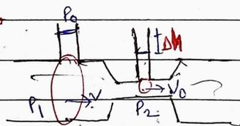
→ The Venturimeter is a device to measure the flow speed of incompressible fluid.
